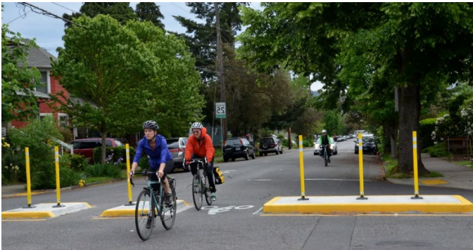
Diagonal diverter with bollards
